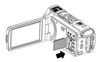
[Insert the memory card directly according to the direction of the chart]
