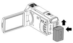
[Install the battery into the camera in the direction of the chart]
